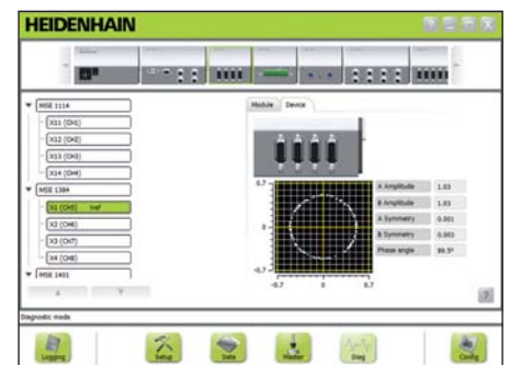
Diagnostics of 1 Vpp signals
