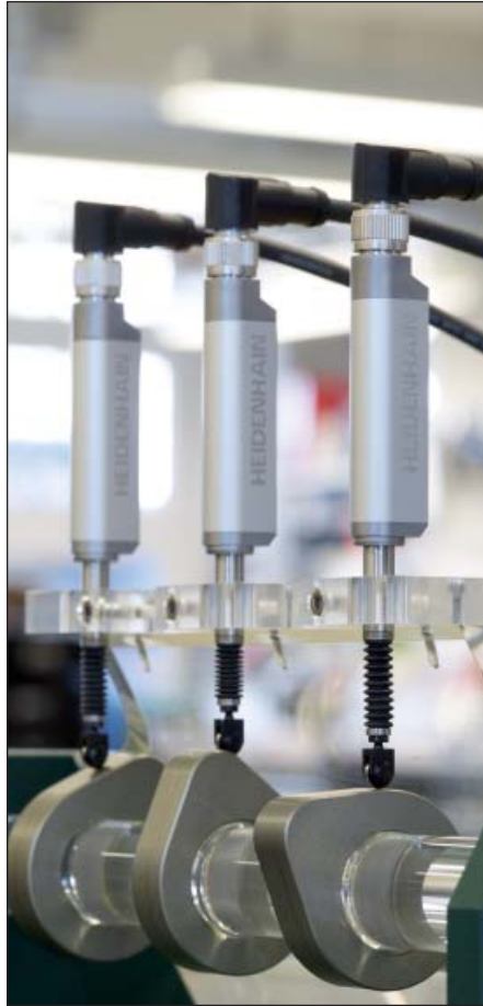
Testing station for flatness inspection
