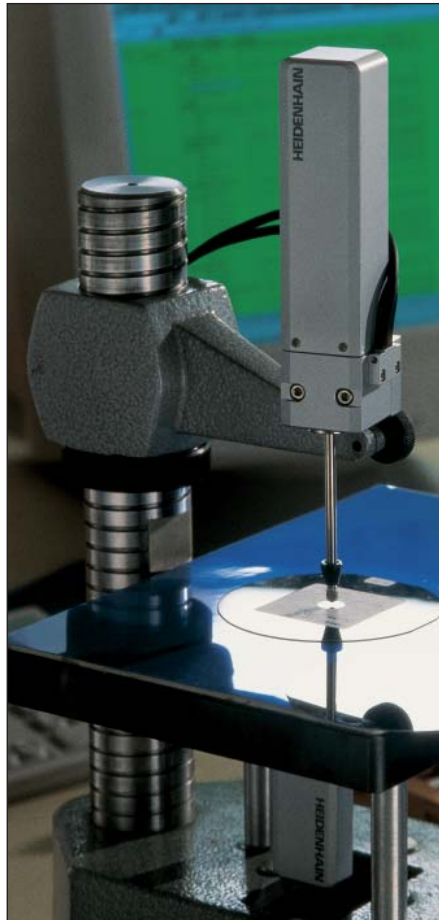
Thickness gauging of silicon wafers
