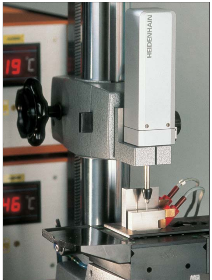
Thickness gauging of silicon wafers
